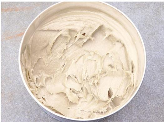
Before applying "Fibreglass Putty," mix the product well to make sure it is smooth.
