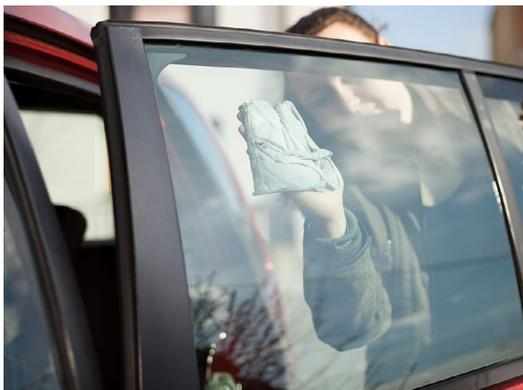
Before applying Antifog, degrease and carefully clean the surfaces to be treated, such as glass and rear-view mirrors. Use the non-woven cloth (TNT) included in the kit to remove dust and dirt. Furthermore, it is important to ensure that the surfaces are dry and free of traces of detergents.
