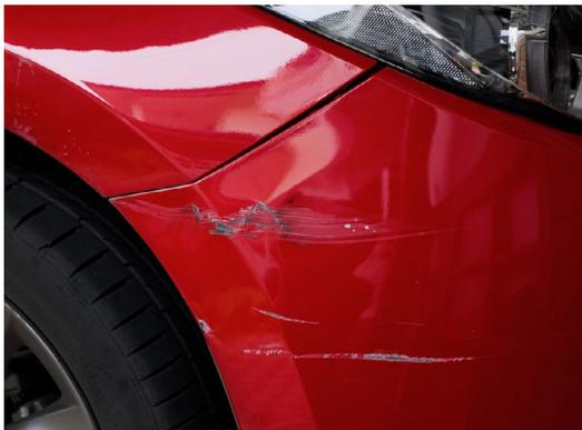
As with any repair process, initial preparation is essential. Start by thoroughly cleaning the damaged surface with a high-quality degreasing cleaner.
